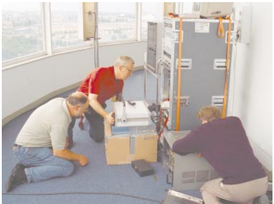
Testing the link termination and DVB-T transmission equipment for the demonstration at IBC 96.
