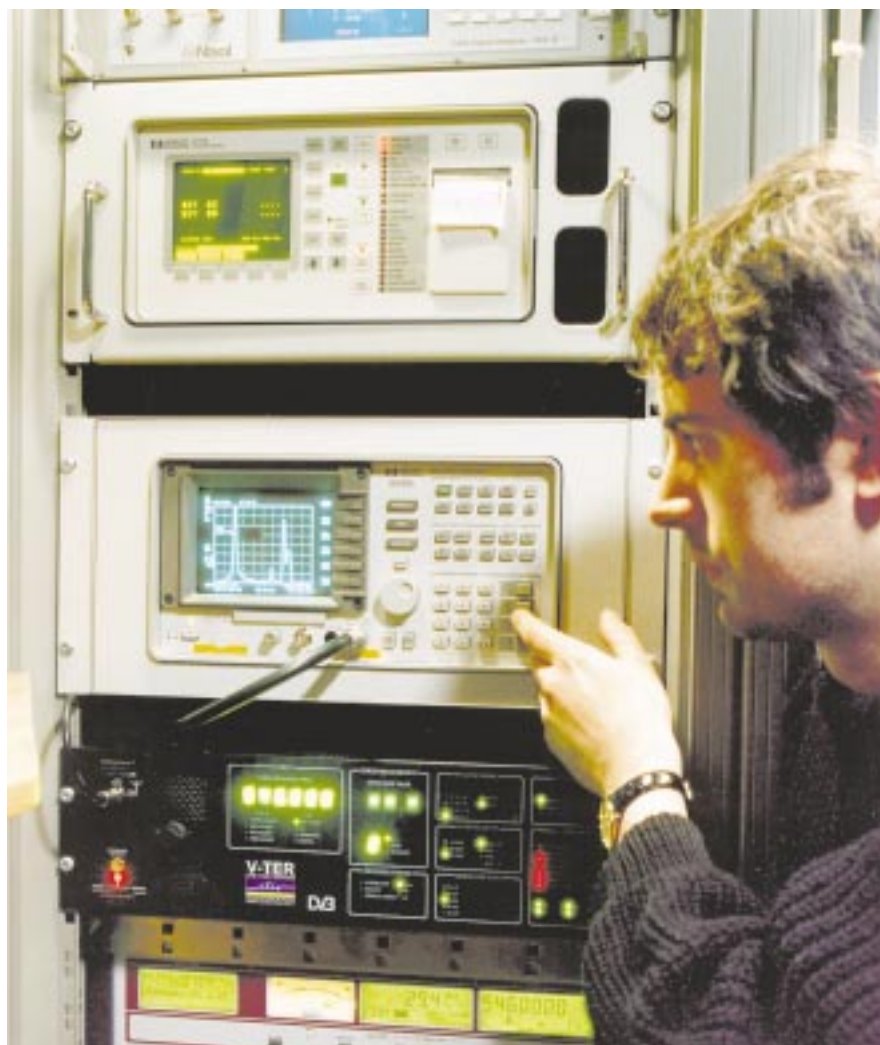
Channel profile in SFN being tested by RTÉ and ITIS in Ireland.
